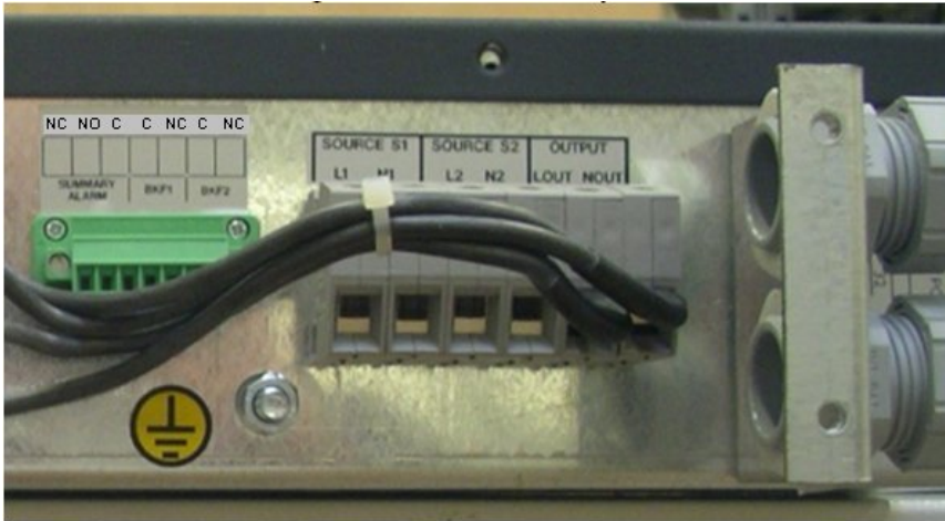
Fig. 9 – Power and signal terminals (cover removed)
