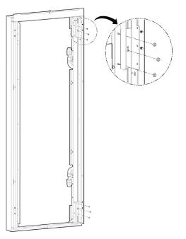
10. With hardware of bag 3, screw (without tightening) the M4 screws with washers starting from the side (3), following on the bottom (3) and then on the top (3). Once, all screws are placed, full tight them to prevent the frame from twisting.
