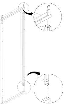
3. Remove the Roof Panel plastic covers on the rack, then install the Cable Pass Through Brushes.
