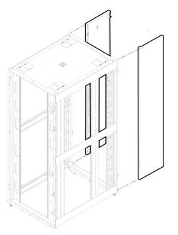
7. With hardware of bag 2, mount the DCD Adapter frame onto the VR Rack. Insert the 8 Torx mounting screws PH M6-1X12mm ZP, using a T30 driver and torque to 10.5 N-m (7.74 ft-lb), then insert and torque the Hex head serrated screw M8X14 (ground screw) to 25.46 N-M (18.78 ft-lb) both.
