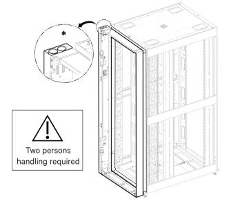
11. From DCD box, use the M5 nuts to screw both corner brackets as it shows in the image.
