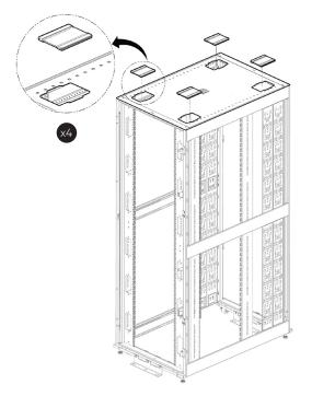
2. Remove the Side Panels (1) to install the Air Recirculation Prevention Kit (2).
