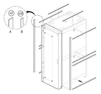
18. Install the VR Networking Rack Bottom Panel.\*\* NOTE: Refer to the VR Networking Bottom Panel Quick Installation Guide for related instructions.
