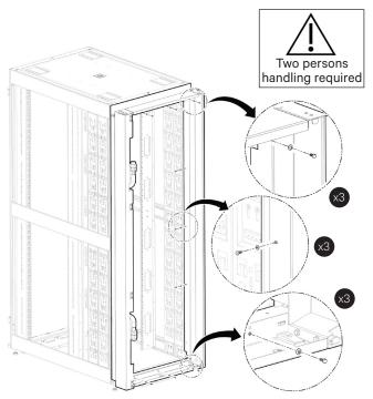
12. Insert and tighten the 2 DCD corner brackets from the DCD box with the hardware included in the DCD. And from hardware of bag 3, insert and tight the M4 screws with washers and ribbed shank rivet as shown below.
