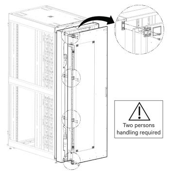
14. Install the DCD swivel-joint covers.
