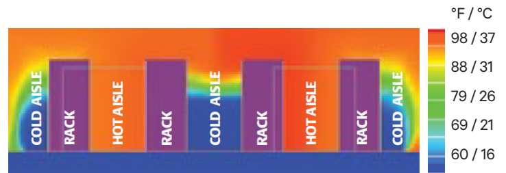
Heat Load = 10 kW Per Rack With Hot Aisle/ Cold Aisle Layout
