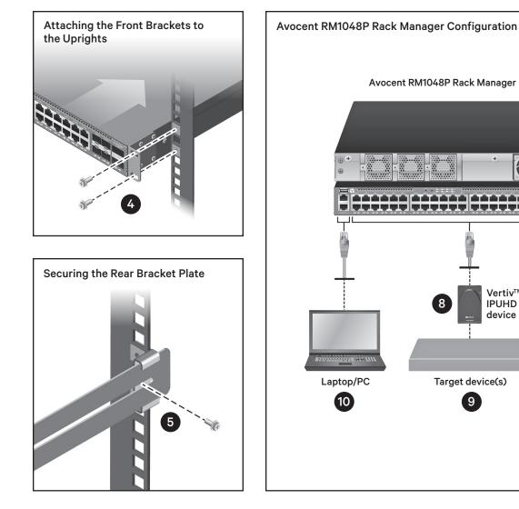
Tighten the screws to firmly secure the rear bracket plate to its rear bracket plate holder.
