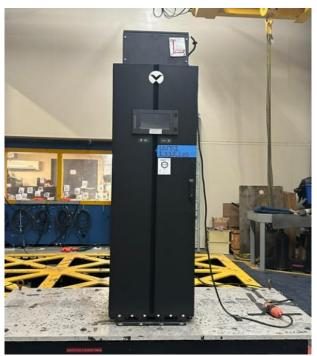
UUT was rigid base mounted to the table using Seismic Kit 570908G1 with (8) 1/2" Grade 8 hex bolts and flat washers.
