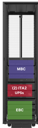
Two UPS Configuration. (9U Maintenance Bypass cabinet requires to be used in this configuration for Vertiv™ Liebert® ITA2 to achieve paralleling for capacity(1+1) or redundancy(2+0)
