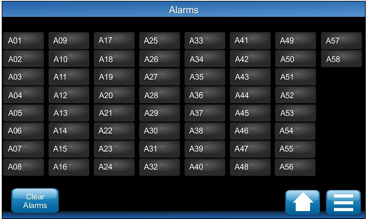
Figure 4.5 Control System Alarms Screen
