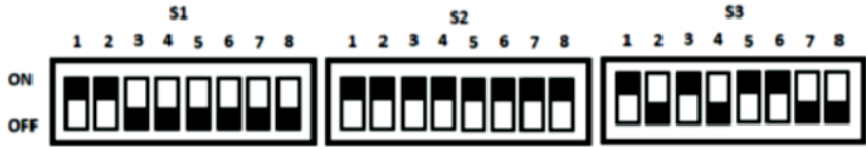
DIP Switches Positions
