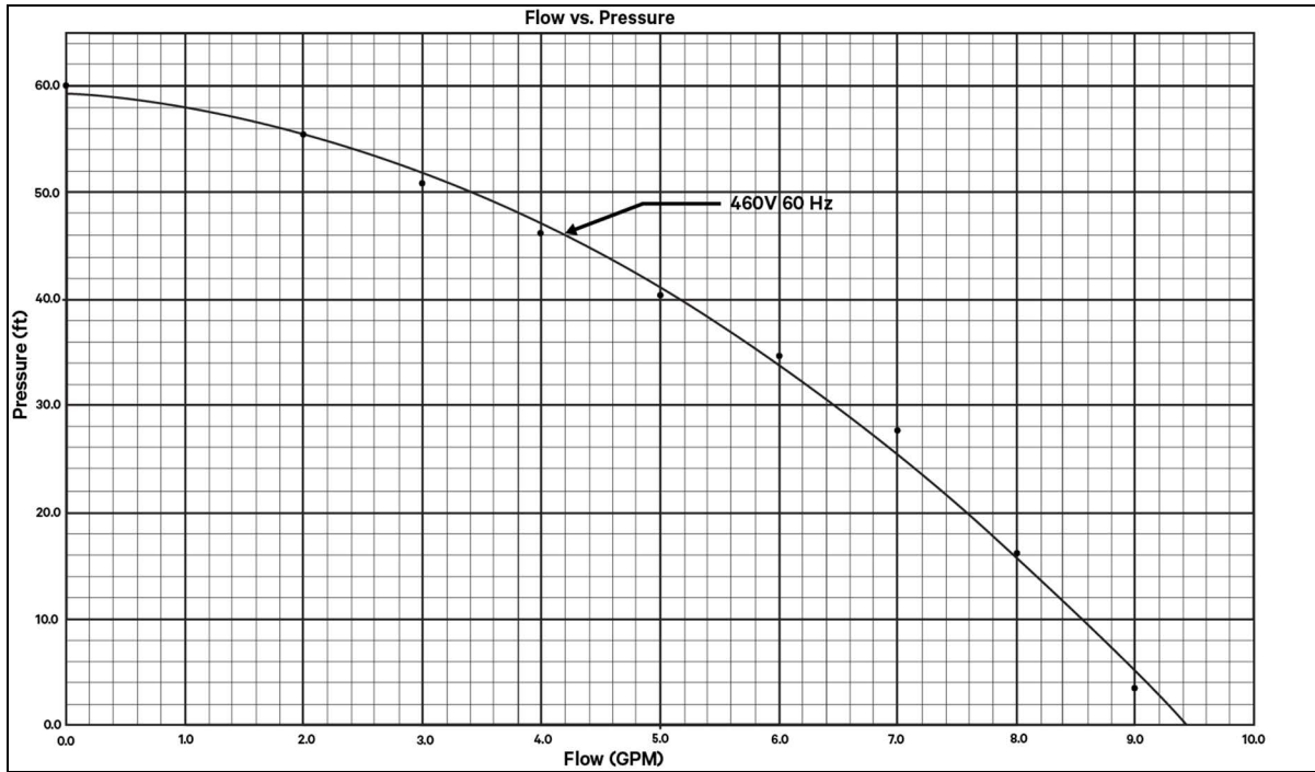
Figure 10.5 Condensate Pump Curve
