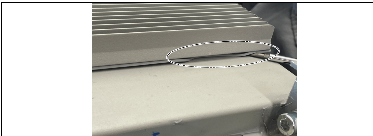
Figure 6.10 Example of Partially Dislodged Gasket
