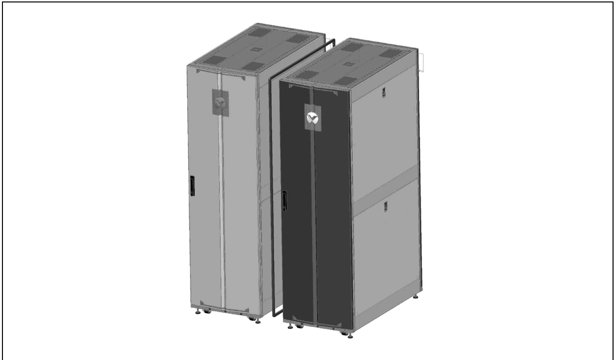
Figure 4.11 Baying gasket location
