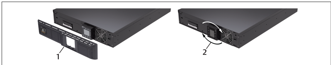
Figure 3.2 Remove the front plastic bezel cover and rotate display
