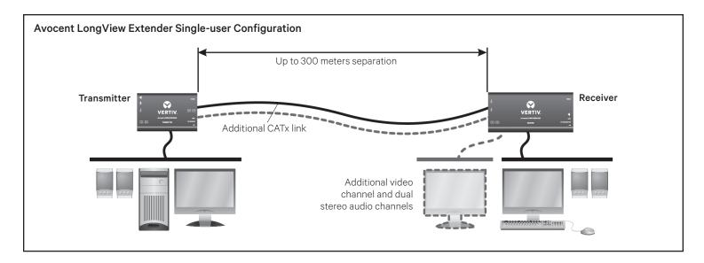
The Avocent LongView high performance KVM extender system provides the fastest way to extend high-quality video, audio and USB data across your network. Transmitter and receivers can be configured in a single-or dual-user configuration to best meet the system needs.
