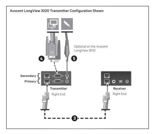
choose to make a secondary connection on the Avocent LongView 3020 extender, that connection is between the top ports.
