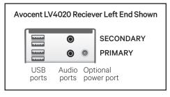
port on the computer to the bottom (primary) DVI-D port on the receiver. Then, connect the video cable from the secondary video port on the computer to the top (secondary) DVI-D port on the receiver.
