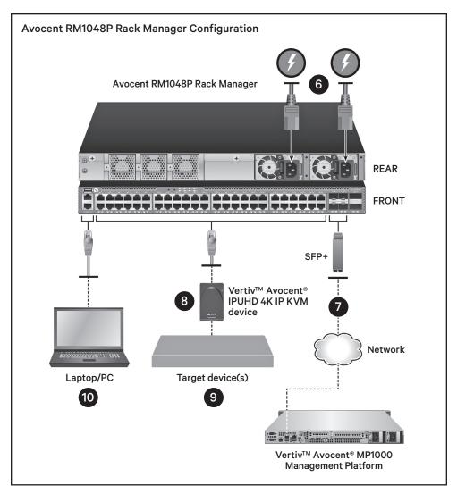
both Power Supply Unit (PSU) ports on the right rear of the rack manager. Verify power by checking the PSU LEDs. The PSU1/PSU2 LEDs illuminate green in normal operation.
