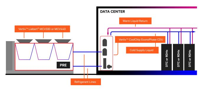
Working in tandem with direct-to-chip cold plates or rear door heat exchangers, the Vertiv™ CoolChip EconoPhase CDU utilizes pumped refrigerant economization (PRE) to eliminate the need for chilled water, allowing you to easily and efficiently cool pods of high-density racks in your air-cooled data center.
