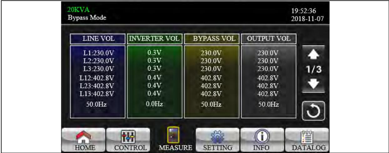
1. **LINE VOL:** The real time value of L1, L2 and L3 phase voltage, L1L2/L2L3/L3L1 voltage and input frequency.
