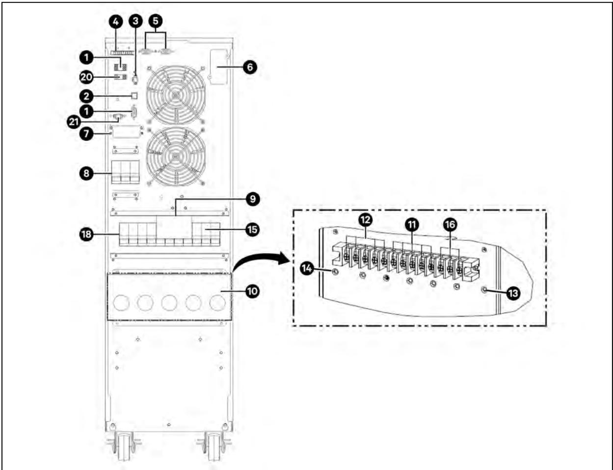
Figure 2.7 HV 40kVA Rear Panel
