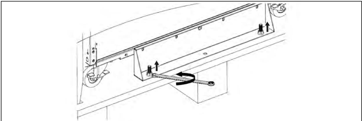
5. To fix the cabinet in position, step on the roller brake and fix the cabinet board to fix the cabinet in place. See **Figure 2.5** on the facing page .
