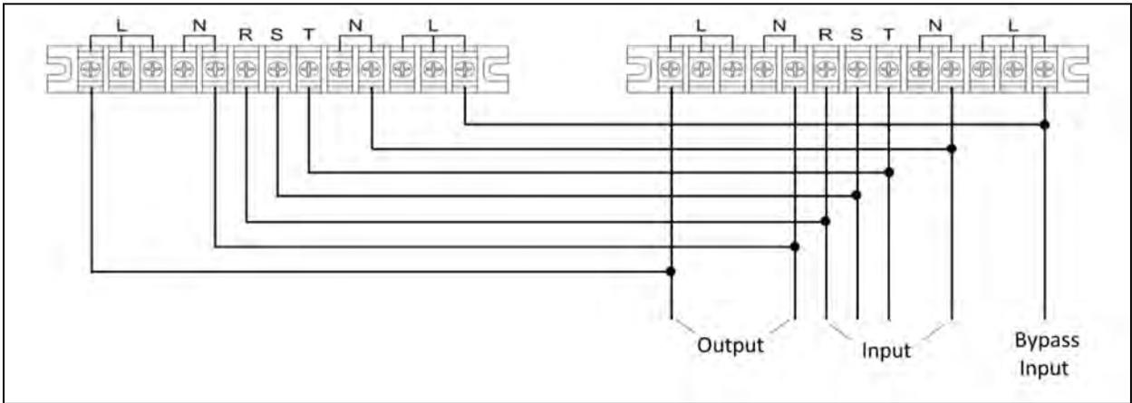
Figure 2.21 Wiring Diagram of Parallel System for HV 40kVA
