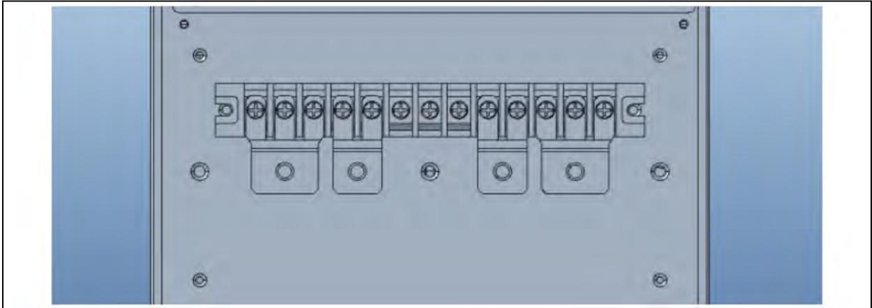
8. Connect the power lines according to the Figure 2.17 below .
