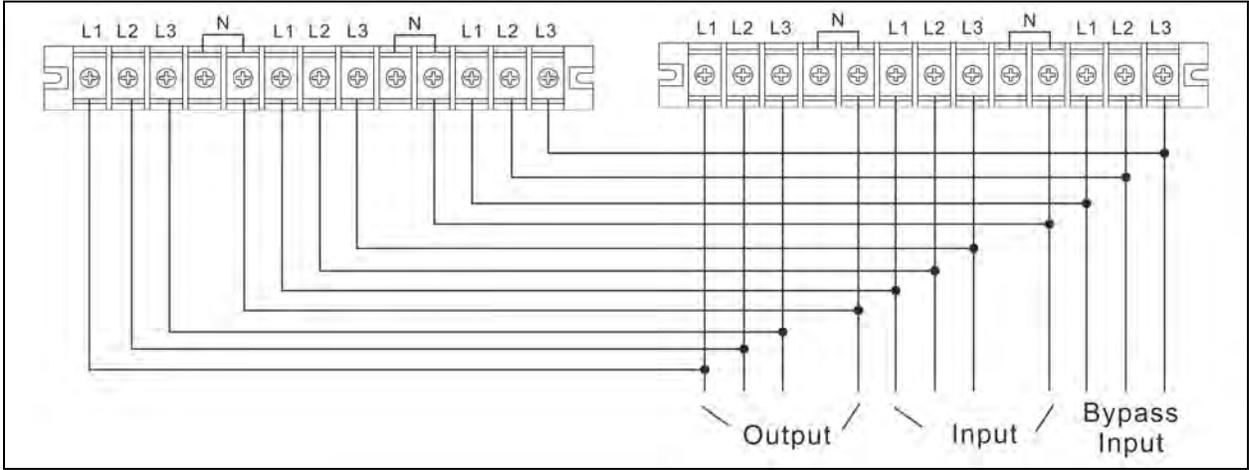
Figure 2.20 Wiring Diagram of Parallel System for 10-15-20kVA with 3-In 1-Out configuration
