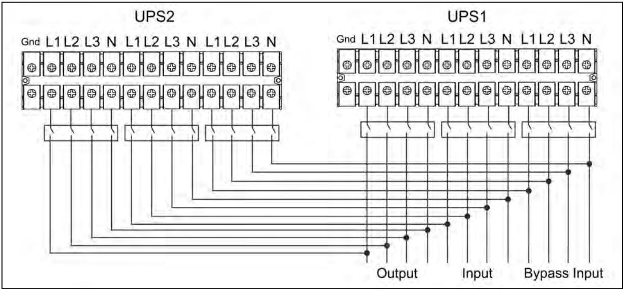
Figure 2.22 Wiring Diagram of Parallel System for HV 80kVA
