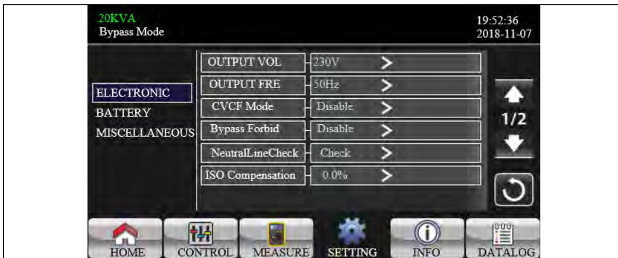
1. **Output VOL:** Select the output rated voltage.
