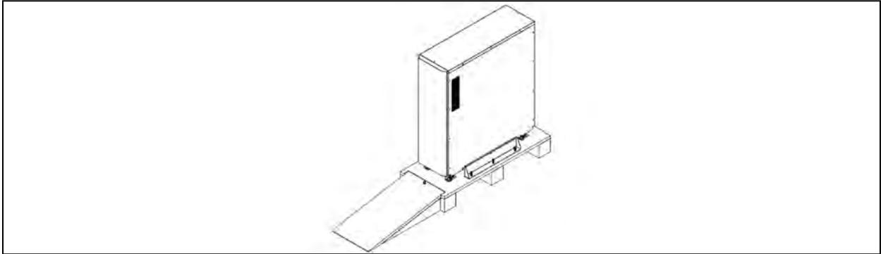
4. Remove two fixing cabinet plates and move the cabinet from the pallet. See **Figure 2.4** below .
