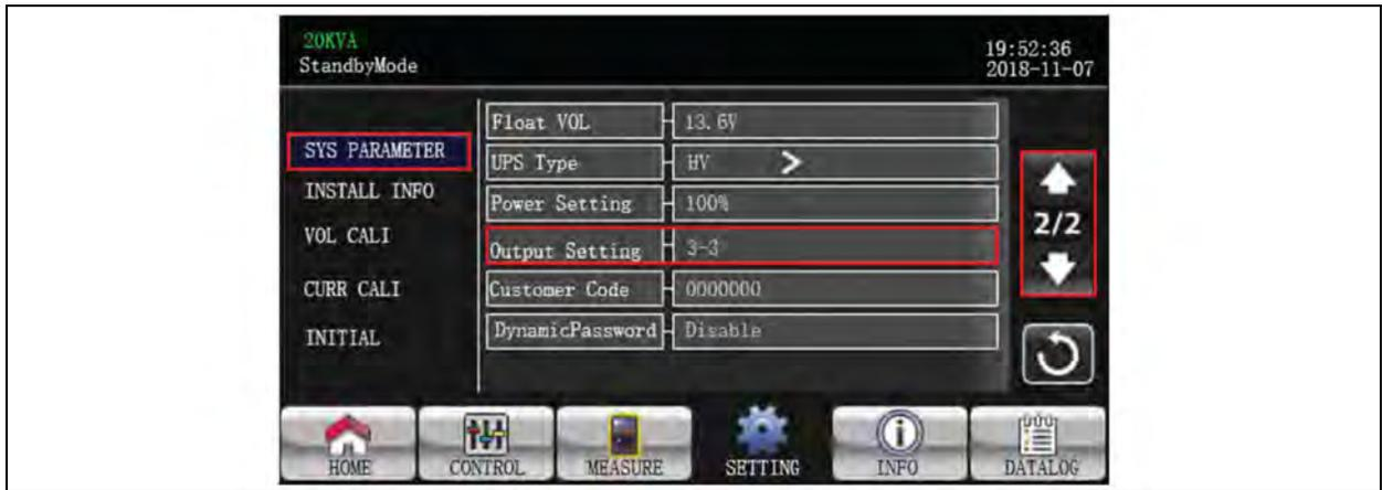
**NOTE:** The 3-1 parameter settings will be saved only when UPS shutdown normally with battery connected.
