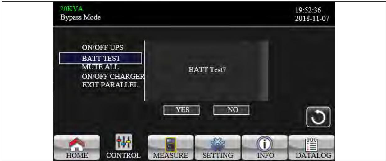
Figure 3.16 Cancel Battery Test Screen
