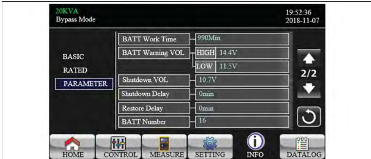
1. **BATT Work Time:** The maximum discharge time in battery mode.
