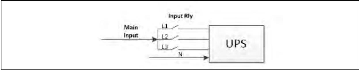
Figure 1.2 Input Relay Diagram for Dual-input Mode
