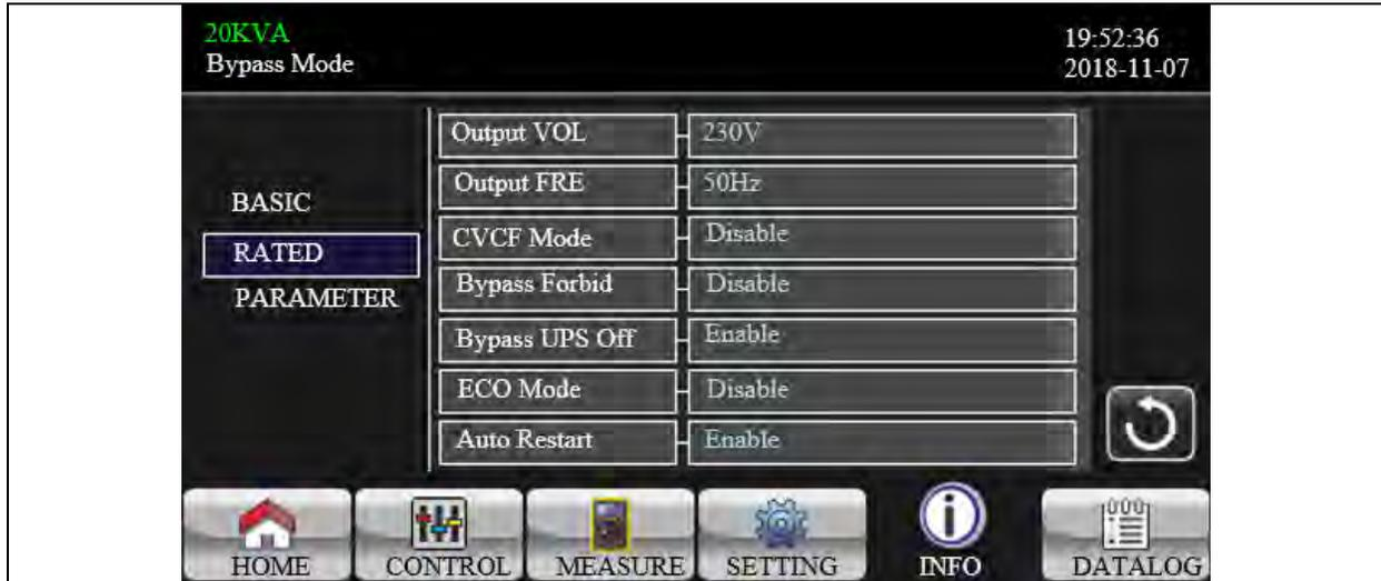
1. **Output VOL:** It shows output rated voltage.
