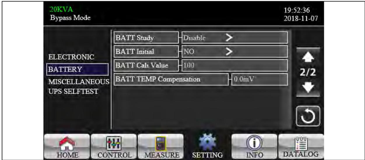
1. **Battery Study:** When battery aging occurs, this function is to calibrate backup time estimation. It's a self-learning function for battery. Currently, this function is not available.
