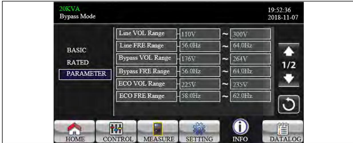
1. **Line VOL Range:** The acceptable line input voltage range.
