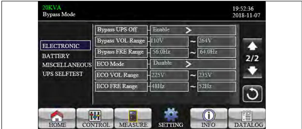
1. **Bypass UPS off:** Select the bypass status when manually turning off the UPS. This setting is only available when “Bypass forbid” is set to “Disable”.
