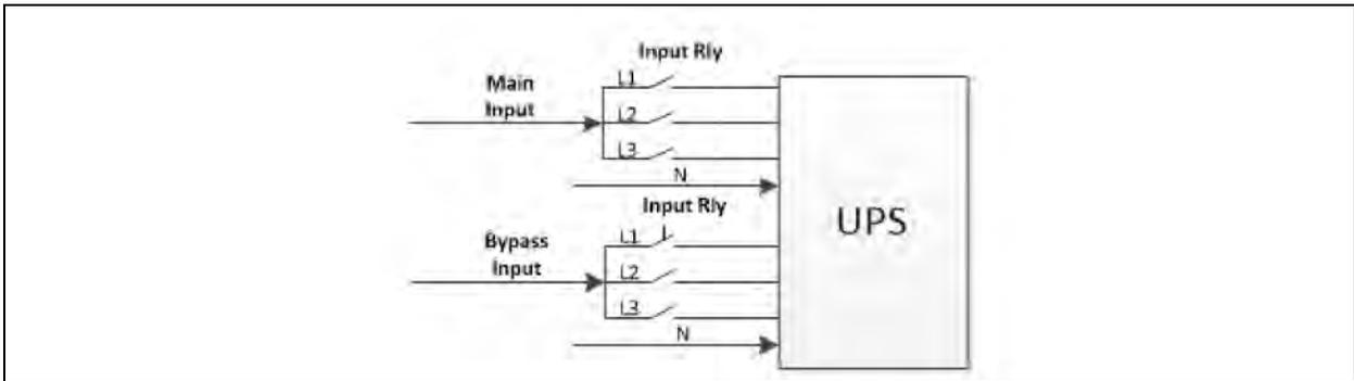
This UPS should be connected with TN grounding/earthing system.
