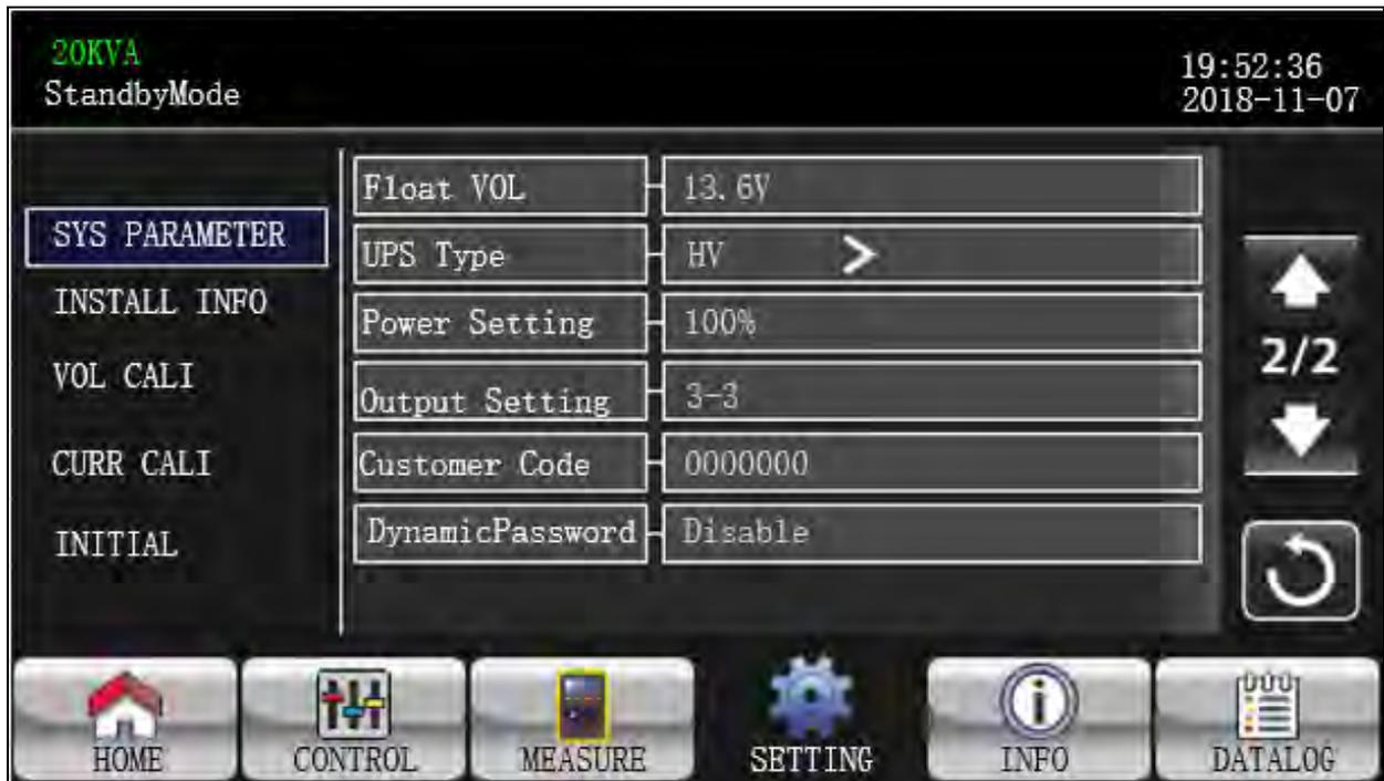
1. **Float VOL:** The setting point of battery float voltage. 13.6V is default setting.
