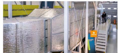
Dedicated area to test the state-of-the-art Liebert EFC - Vertiv's highly efficient indirect evaporative freecooling unit. Testing parameters include IT loads of up to 450 kW and an airflow of up to 120,000 m<sup>3</sup> per hour at any external ambient temperature required to simulate typical peak conditions across the EMEA region.
