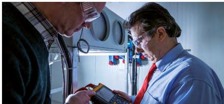
Designed for conditioners belonging to the Telecom sector, the Research & Development Validation Lab 2 includes two different testing chambers: one simulating internal ambient conditions from 0°C to 60°C and the other simulating external ambient conditions from -32°C to 60°C. This validation area can balance a thermal load of up to 100 kW (50 kW in each room).
