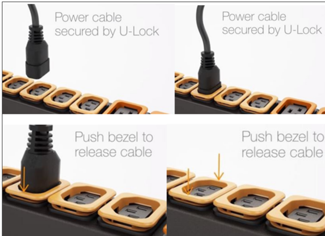
Figure 2.14 U-Lock Cord Retention Operation
