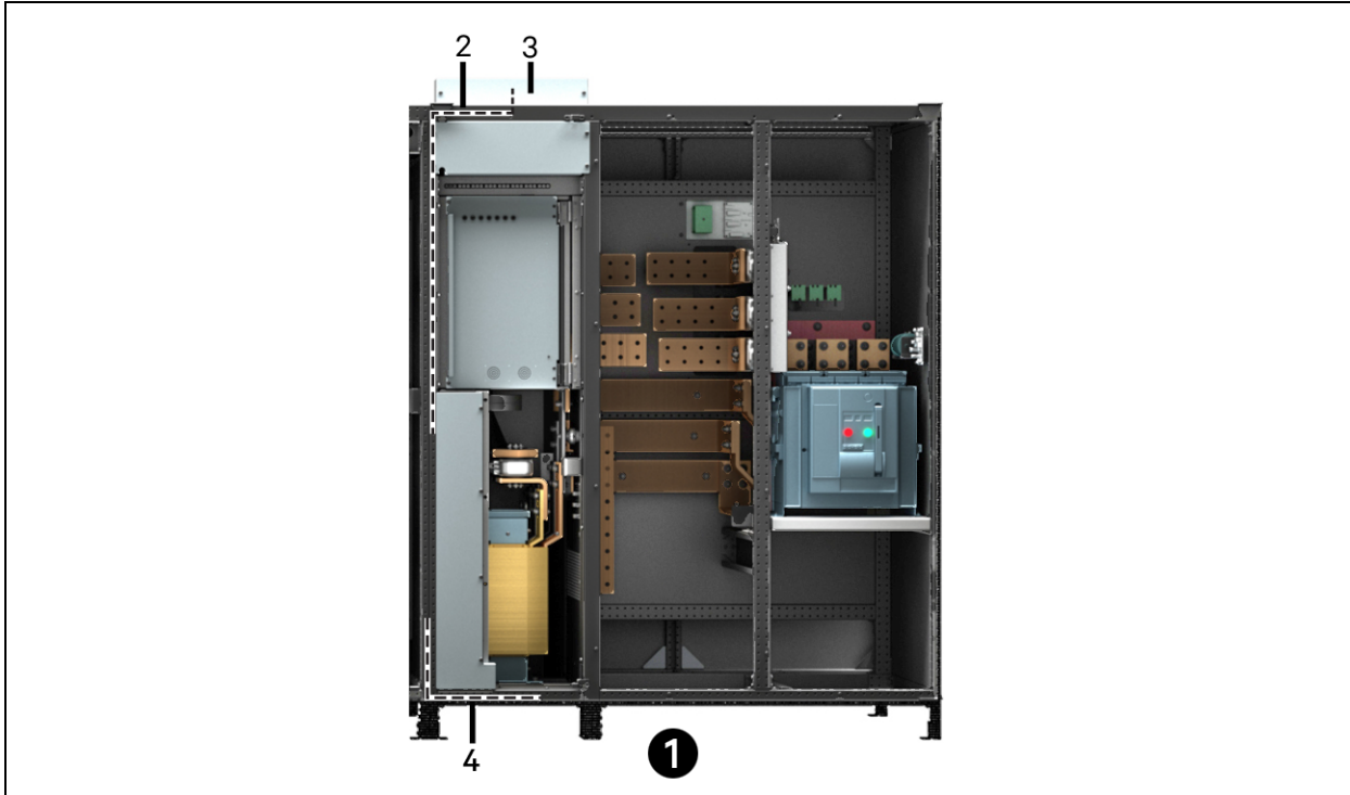
Figure 4.4 Low-Voltage Cable Routing Example
