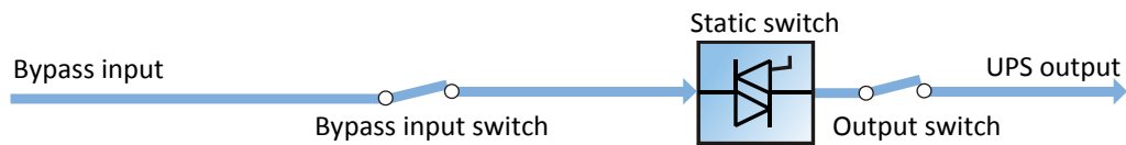
Figure 1-5 Schematic diagram of bypass mode
