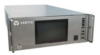
The Vertiv™ CoolChip CDU 100 in-rack coolant distribution unit (CDU) provides effective separation of the facility fluid circuit and secondary fluid network via a liquid-to-liquid heat exchanger for single rack direct-to-chip cooling applications.
