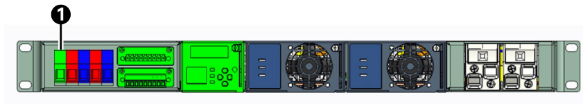
Figure 5.1 Earthing Connection on the Front Side
