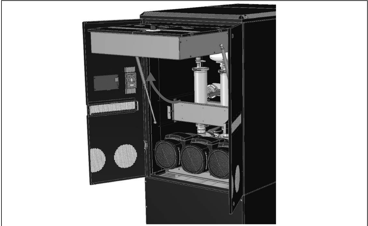
Figure 5.1 Access to Secondary Filters with Electrical Panel in Horizontal Position
