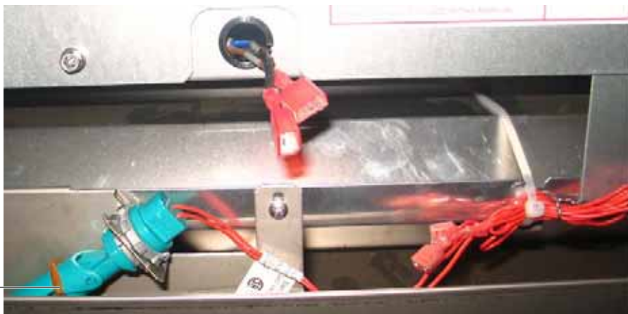
Figure 2-38 Floating pole of high water-level switch
