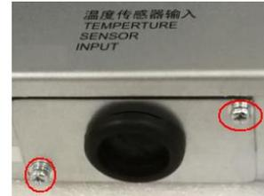
Figure 2-14 Loosening the fixing screw
