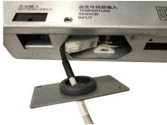
Figure 2-17 Connecting the terminal
