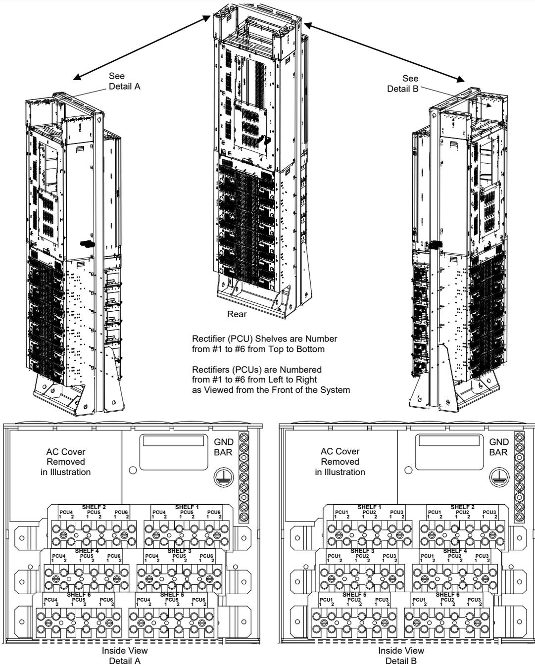
Connections to Optional List 46 Top Mount AC Input Termination Panel (Three-Phase)
