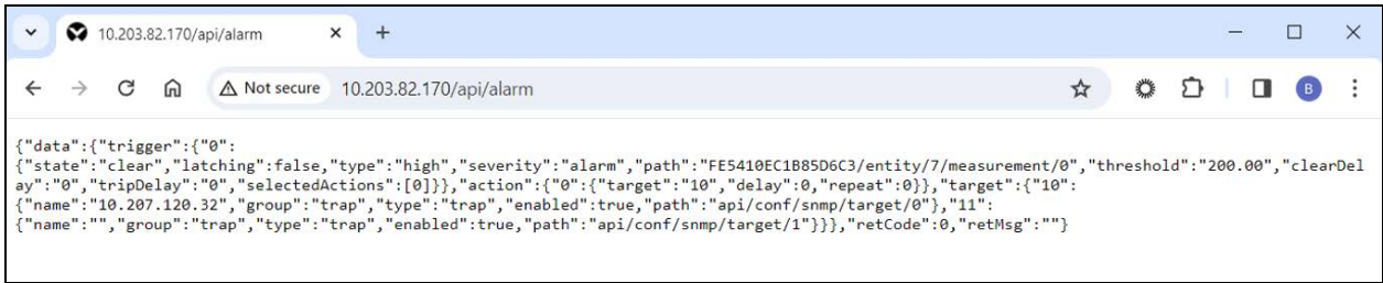
Figure 10.29 Extract Alarm Configuration
