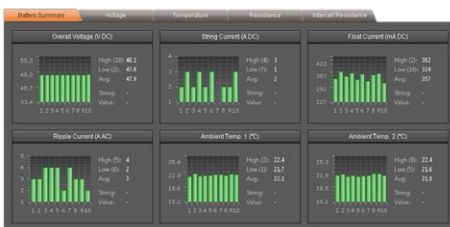
View data on parallel battery strings simultaneously.
