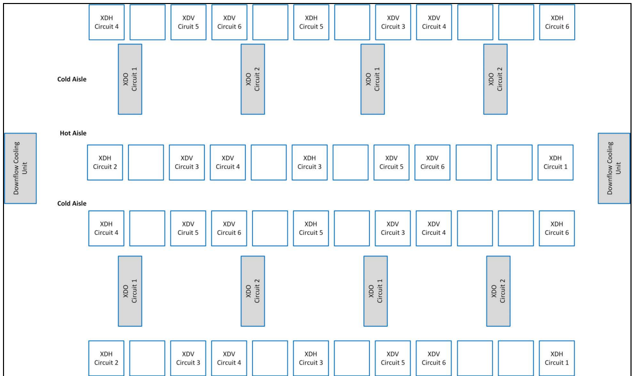
Figure 3.10 Multiple Liebert® XD Modules in an Interlaced System
