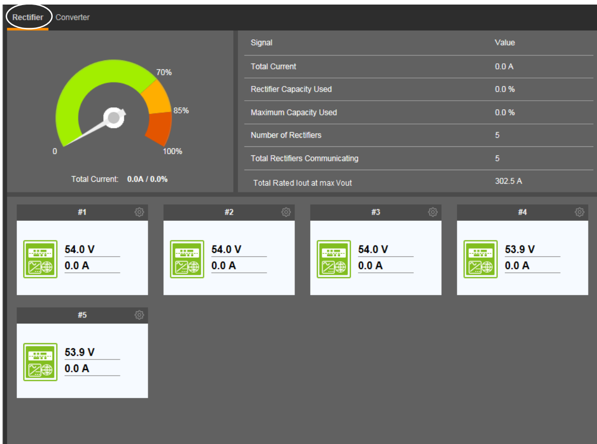
Figure 5.10 Rectifier Device Group Status Page Tab
