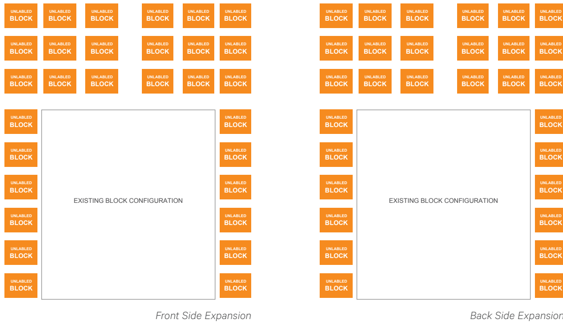
Figure 11b – Block Layout [2400D to 5400D], 300-pair grills (1 x 6) and 450-pair grills (3 x 3)
