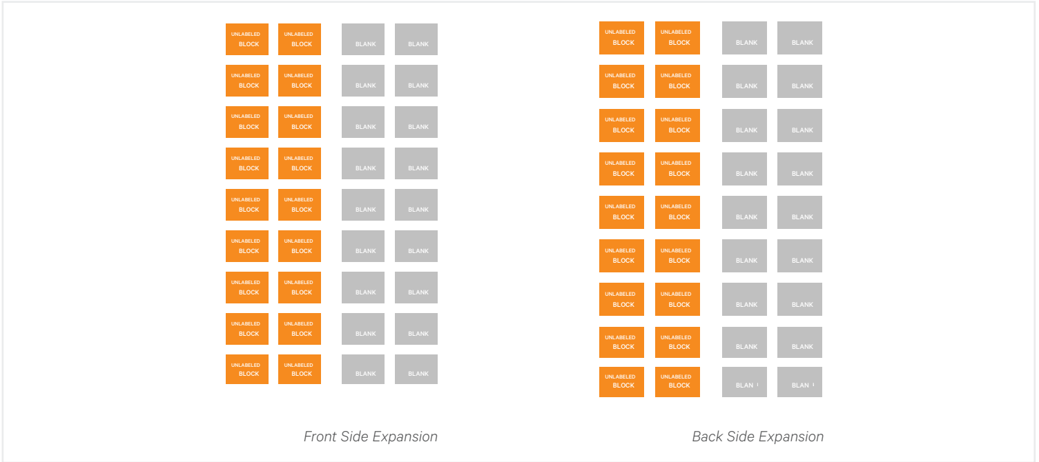
Figure 27d – Block Layout [40-Type Series, 3600D to 5400D, 900-pair grills (2 x 9)]
