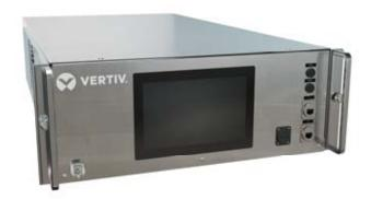
The Vertiv<sup>™</sup> CoolChip CDU 100 in-rack coolant distribution unit (CDU) provides effective separation of the facility fluid circuit and secondary fluid network via a liquid-to-liquid heat exchanger for single rack direct-to-chip cooling applications.
