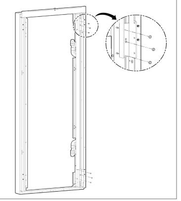
12. Insert and tighten the 2 DCD corner brackets from the DCD box with the hardware included in the DCD. And from hardware of bag 3, insert and tight the M4 screws with washers and ribbed shank rivet as shown below.
