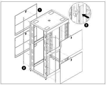
3. Remove the Roof Panel plastic covers on the rack, then install the Cable Pass Through Brushes.
