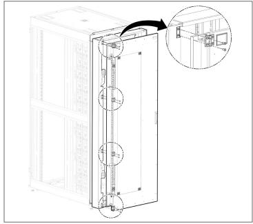
14. Install the DCD swivel-joint covers.
