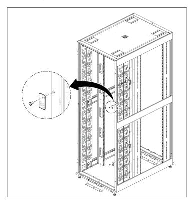
7. With hardware of bag 2, mount the Vertiv<sup>™</sup> DCD Adapter frame onto the VR Rack. Insert the 8 Torx mounting screws PH M6-1X12 mm ZP, using a T30 driver and torque to 10.5 N-m (7.74 ft-lb), then insert and torque the Hex head serrated screw M8X14 (ground screw) to 25.46 N-m (18.78 ft-lb) both.
