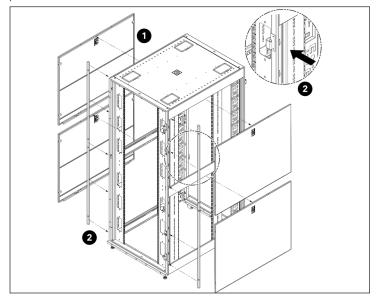
3. Remove the Roof Panel plastic covers on the rack, then install the Cable Pass Through Brushes.
