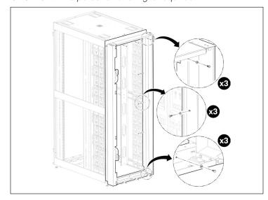
11. From DCD box, use the M5 nuts to screw both corner brackets as it shows in the image.
