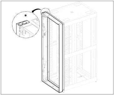
10. With hardware of bag 3, screw (without tightening) the M4 screws with washers starting from the side (3), following on the bottom (3) and then on the top (3). Once, all screws are placed, full tight them to prevent the frame from twisting.
