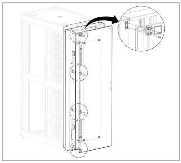
14. Install the DCD swivel-joint covers.
