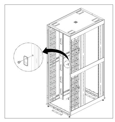
7. With hardware of bag 2, mount the Vertiv™ DCD Adapter frame onto the VR Rack. Insert the 8 Torx mounting screws PH M6-1X12 mm ZP, using a T30 driver and torque to 10.5 N-m (7.74 ft-lb), then insert and torque the Hex head serrated screw M8X14 (ground screw) to 25.46 N-m (18.78 ft-lb) both.
