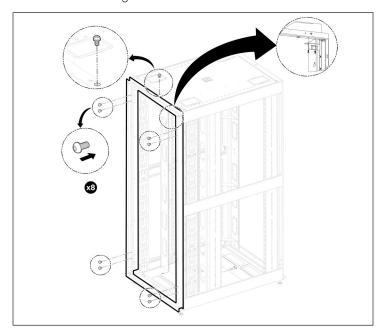
8. Discard unnecessary hardware from the DCD frame. All spring nuts (b), 22xM5x10 screws (a), all washers and 6 diamond nuts (c).
