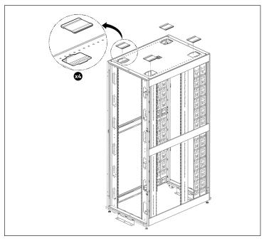
4. Install the EIA rail covers as shown below, by tighten the M6 screws and M6 nuts.
