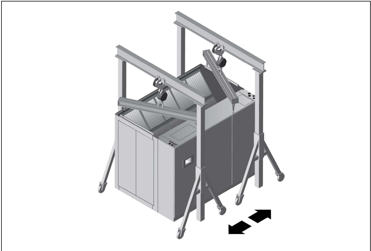
Figure 5.5 Moving the Unit with Rigging
