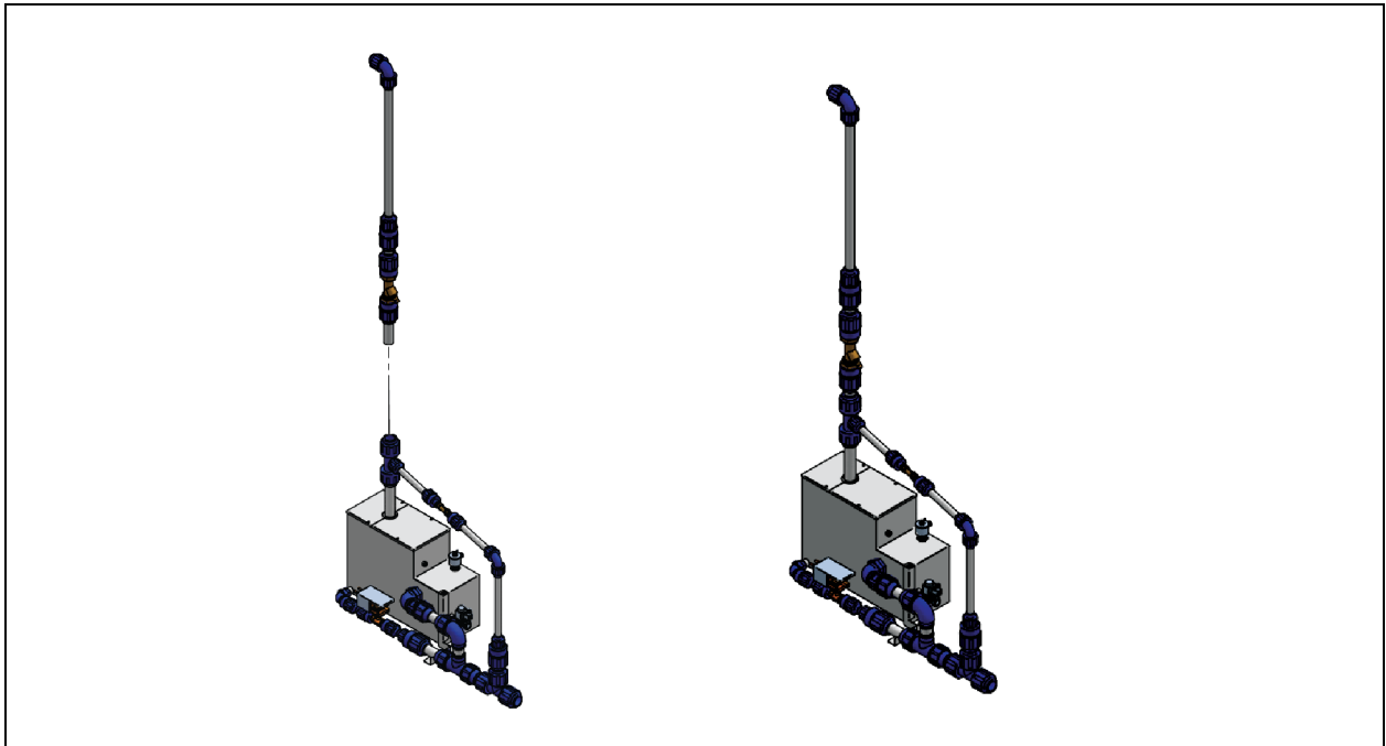
Figure 6.24 Installing the Front Riser Pipe
